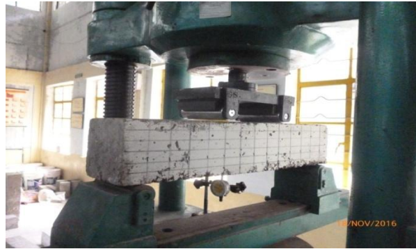
Figure 3: Flexure Test on Beam
